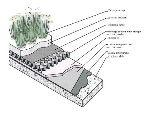
Structure of an extensive green roof
