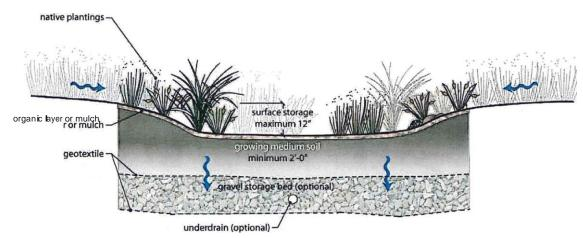
Figure 1: Typical Bioinfiltration Facility
