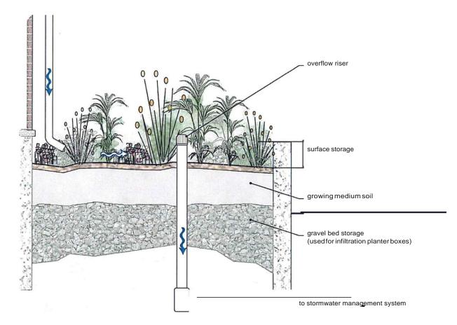
Figure 7: Flow-through Planter Box (Adapted from City of Portland, 2002)
