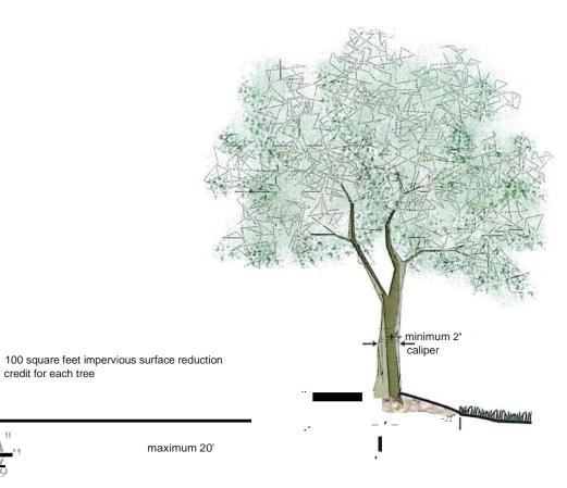
Figure 4: Stormwater Tree
